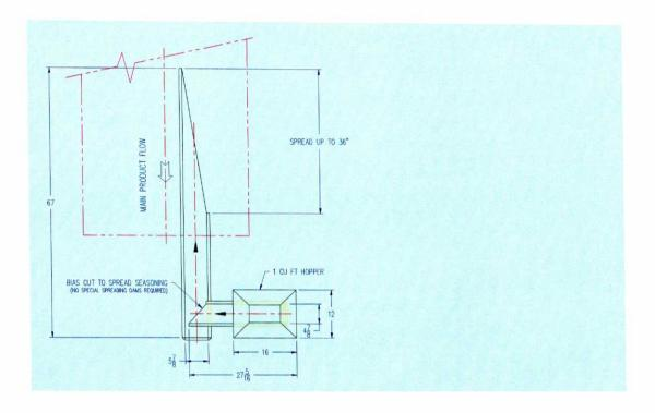
The profile of the conveyor is very low to fit inside the tumbler drum. The frame stays outside whereas the bias cut section of the feeder cantilevers on the inside of the drum to spread seasoning evenly over tumbling product. The drive is easily accessible and is on the infeed end. The isolation mounts minimize vibration transmission to the structure. The construction is all stainless steel including drive components and frame to allow complete wash down.
